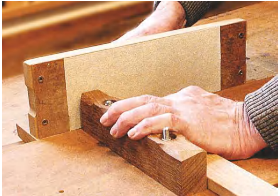
▲ Pic.2 The sanding jig at work on a shooting board; offset pad protects the fence from damage
